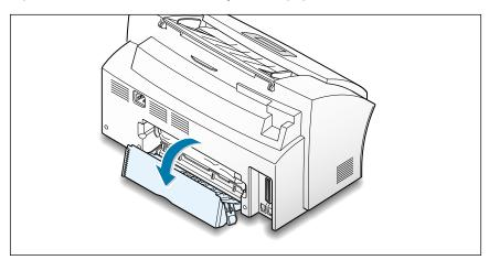
3. Pull the paper carefully out to remove it from the paper path.
